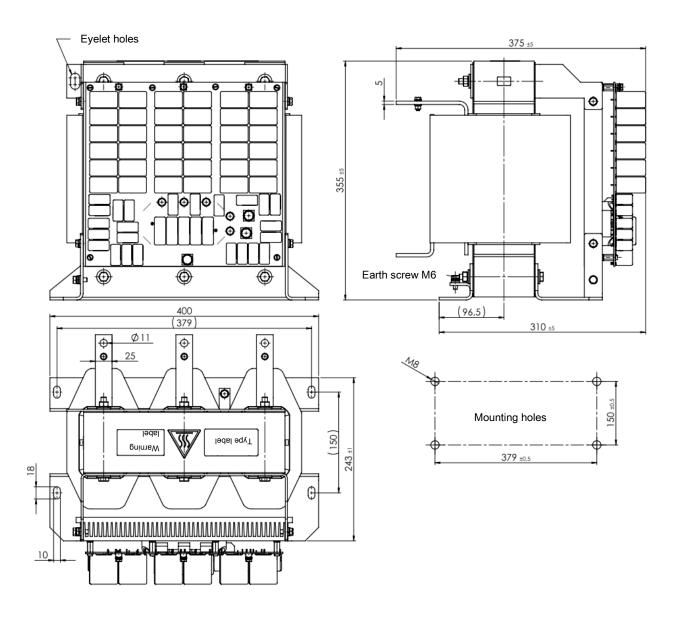
Picture 3-5 Technical drawing dv/dt filter MTZEF051-25
