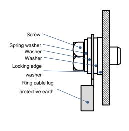
Picture 4-6 Electrical connections dv/dt filter TEF1203-0MB
