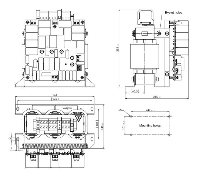
Picture 3-1 Technical drawing dv/dt filter MTZEF051-21
