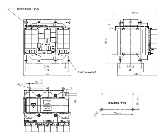
Picture 3-6 Technical drawing dv/dt filter MTZEF051-26
