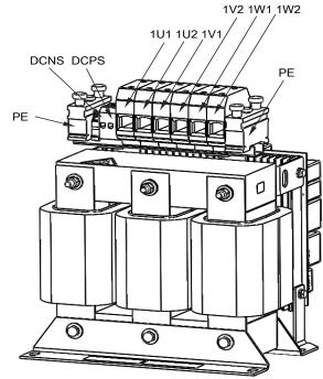
Picture 4-1 Electrical connections dv/dt filter TEF1203-0GB
