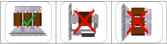
Picture 3-1 Mounting position in the enclosure
