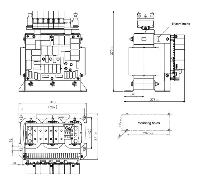
Picture 3-3 Technical drawing dv/dt filter MTZEF051-23
