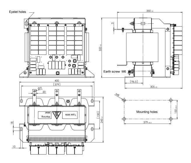
Picture 3-4 Technical drawing dv/dt filter MTZEF051-24
